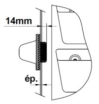
4) Position the VIGIBELT® TOUCH sensors on the openings and tighten the M6 locknuts (torque 4 N.m) according to Diagram-D.
