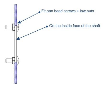
3) Adjust the triggering distance of the VIGIBELT® TOUCH sensors. This distance is the dimension between the inside face of the elevator and the contact face of the sensor.
